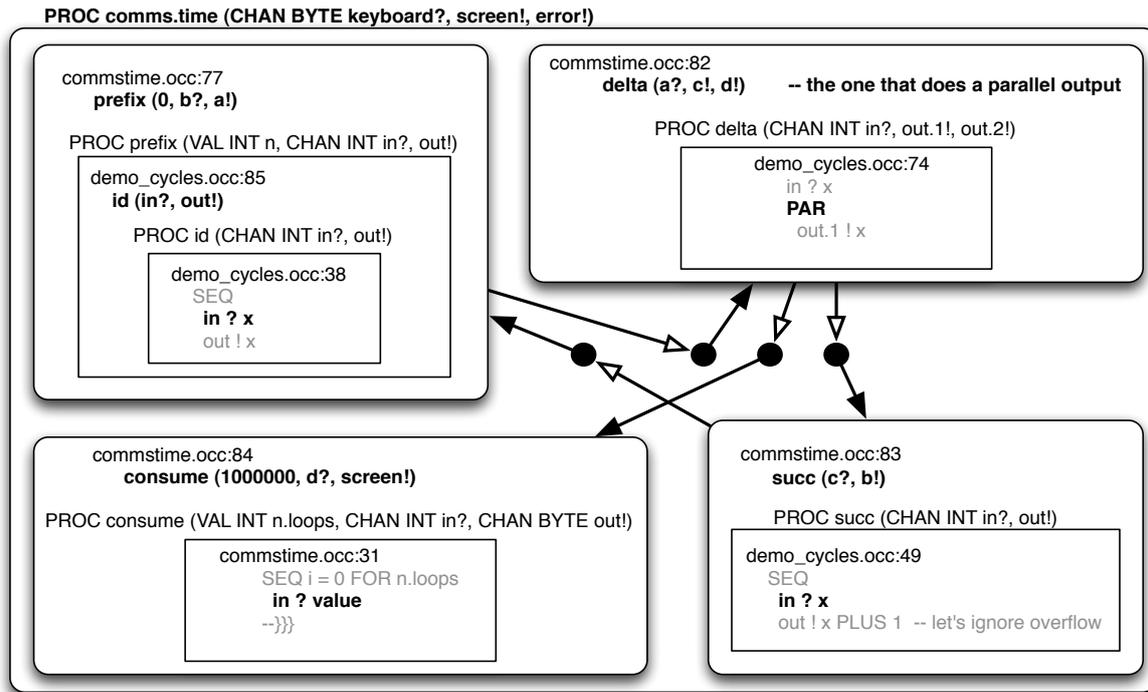
**Figure 1.** Idealised visualisation of commstime.occ. Curved boxes represent processes. Squared boxes represent calls in the call stack. Bold text is the present line being executed, as taken from the source file. Dots are channels, with arrowed lines representing communication requests. Hollow arrows are previously executed input or output, and filled arrows are active blocked requests.
